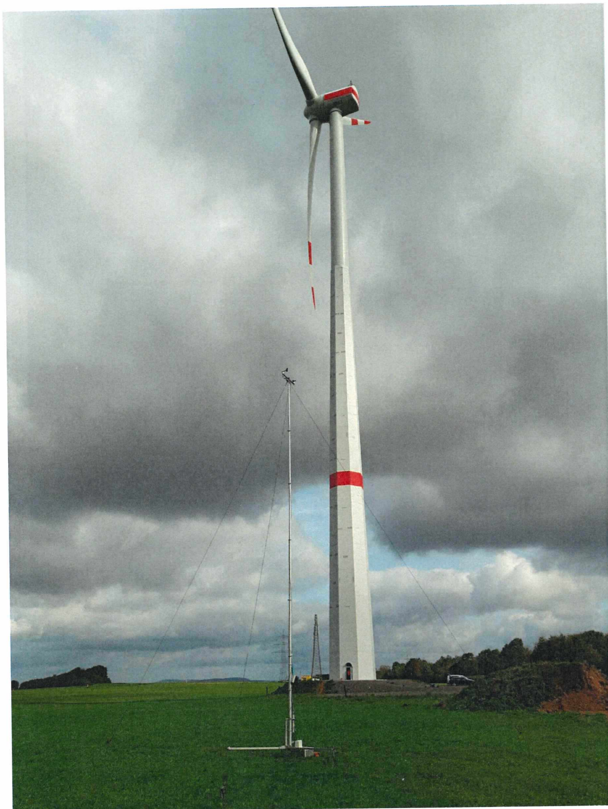
Bild 8-2: 10 m Windmessmast in Relation zur vermessenen WEA
